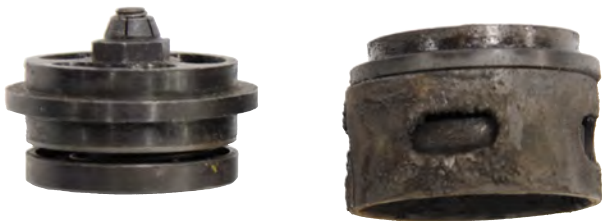
Carbon build-up on disc style valves
